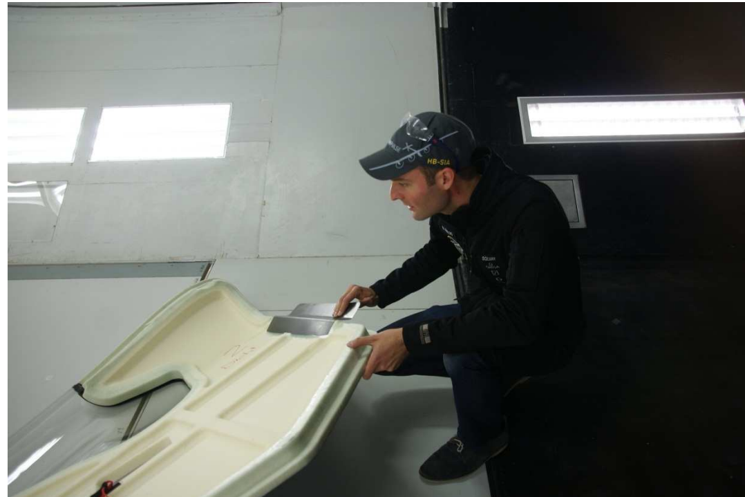
Door with the hinge made of a PU-carbon fibre composite
